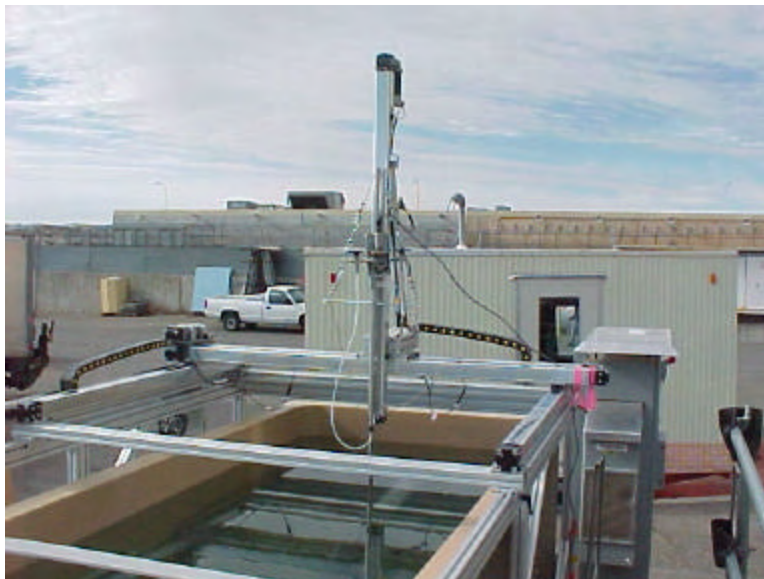
Figure 3.4. Gantry used to collect velocity measurements in the test facility.
