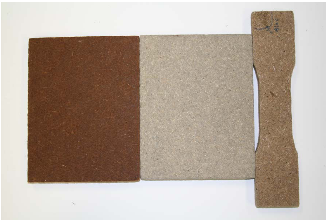
Figure 1: From Left to Right. Hardwood-based Celotex™ from Sunbury Plant, Softwood-based Celotex™ from Danville Plant, and Cane-based Celotex™ from Marrero Plant.
