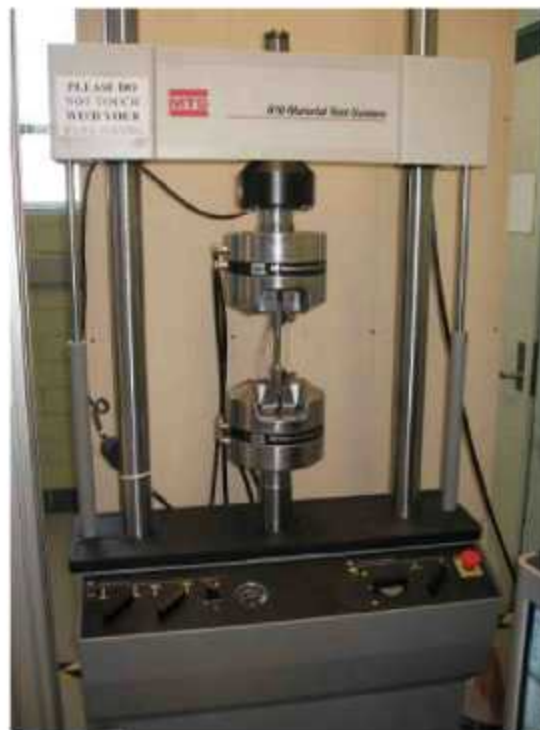
Figure 59. Fatigue test setup.
