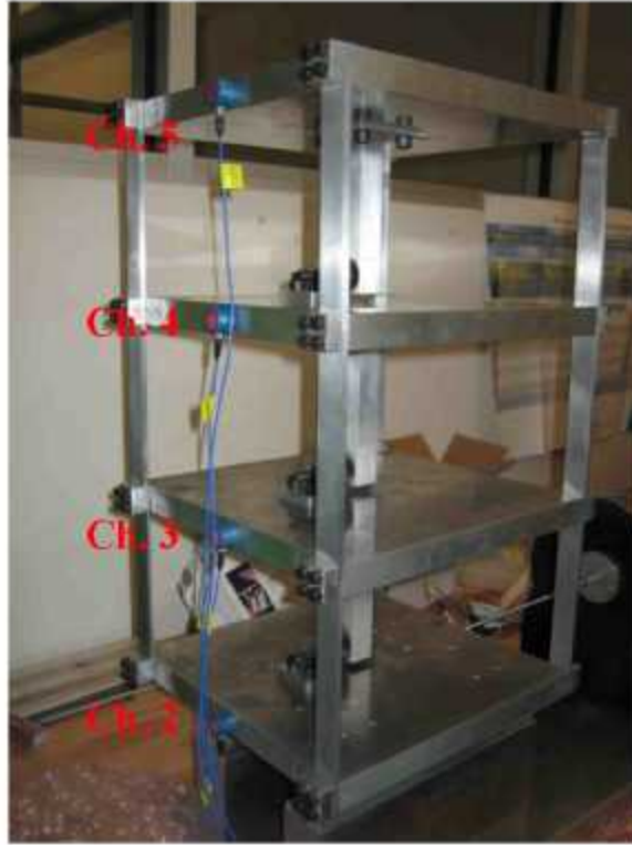
Figure 93. Attachment of accelerometers.
