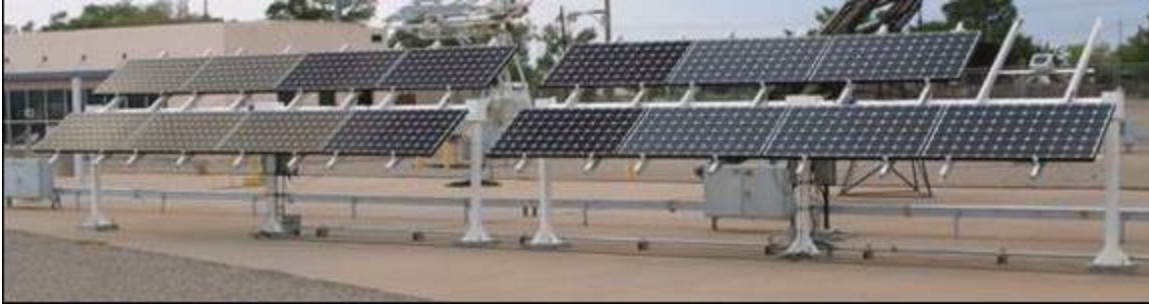
Figure 2.8-1: Field testing of modules with various ARC glass at Sandia National Laboratories.
