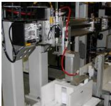
Figure 2.10-2: Wafer gripper used for cell stringing
