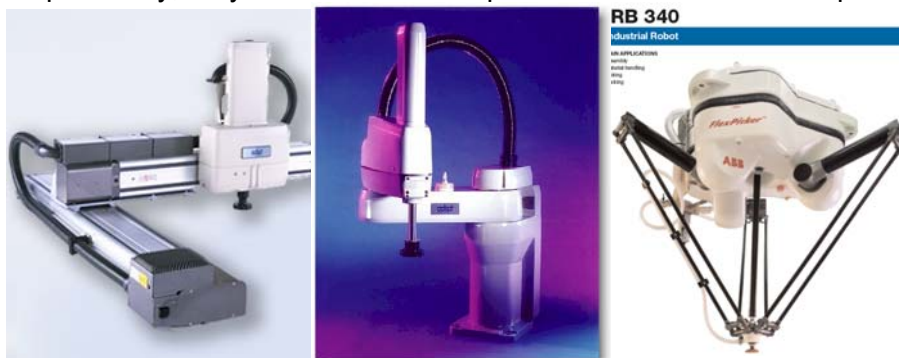
Figure 2.2-1: Left to right: Cartesian, SCARA, and parallel robots
