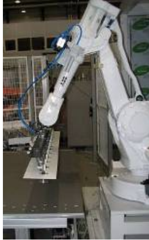
Figure 2.10-3: Robot for string handling
