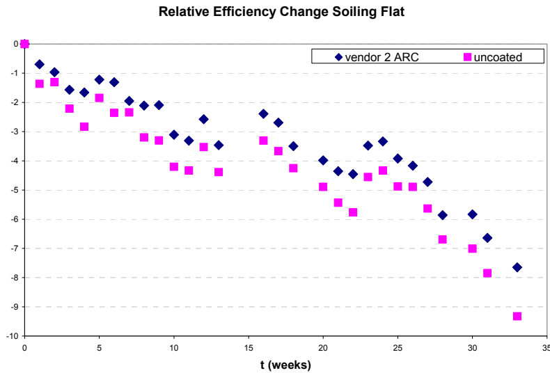
Figure 2.14-2: Soiling test results of AR coated glass and non-AR coated glass
