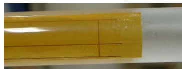
Figure 3: One turn measuring coil printed on a flexible circuit sheet glued on a quartz rod.
