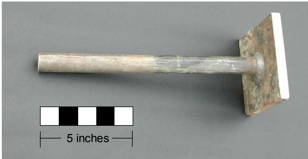
Figure 2.4. Extraction Plate Used to Remove Geoprobe® Rod from the Ground During Aquifer Tube Installation
