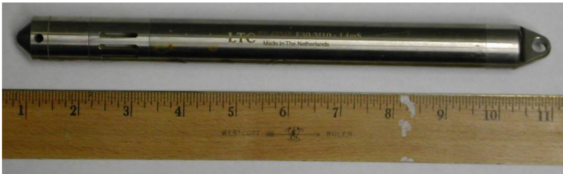
Figure 2.5. Continuous Data Loggers from Solinst Canada, Ltd.
