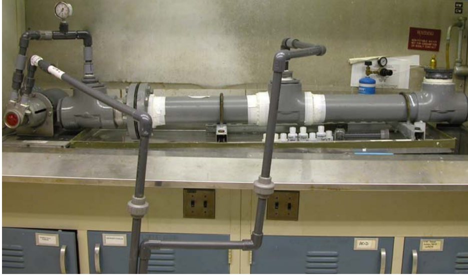
Figure 2. Full-Scale Coalescer Test Unit
