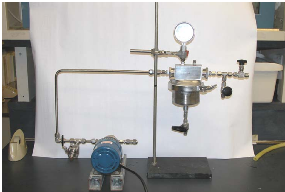
Figure 1. Bench-Scale Coalescer Unit
