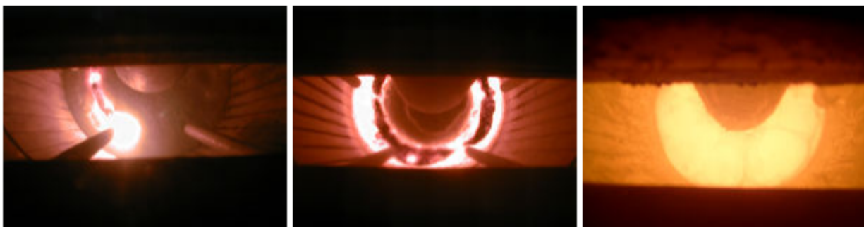
(a) Ignition of Ti Ring (b) Completion of Ignition (c) Preparation of Glass Melt Figure 3. Initial Melting of Glass in CCIM Using a Titanium Susceptor
