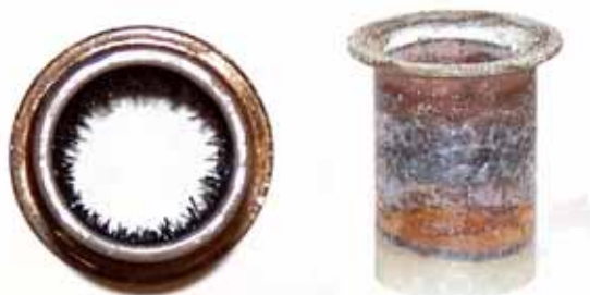
Figure 6 Offgas Line Showing Deposits
