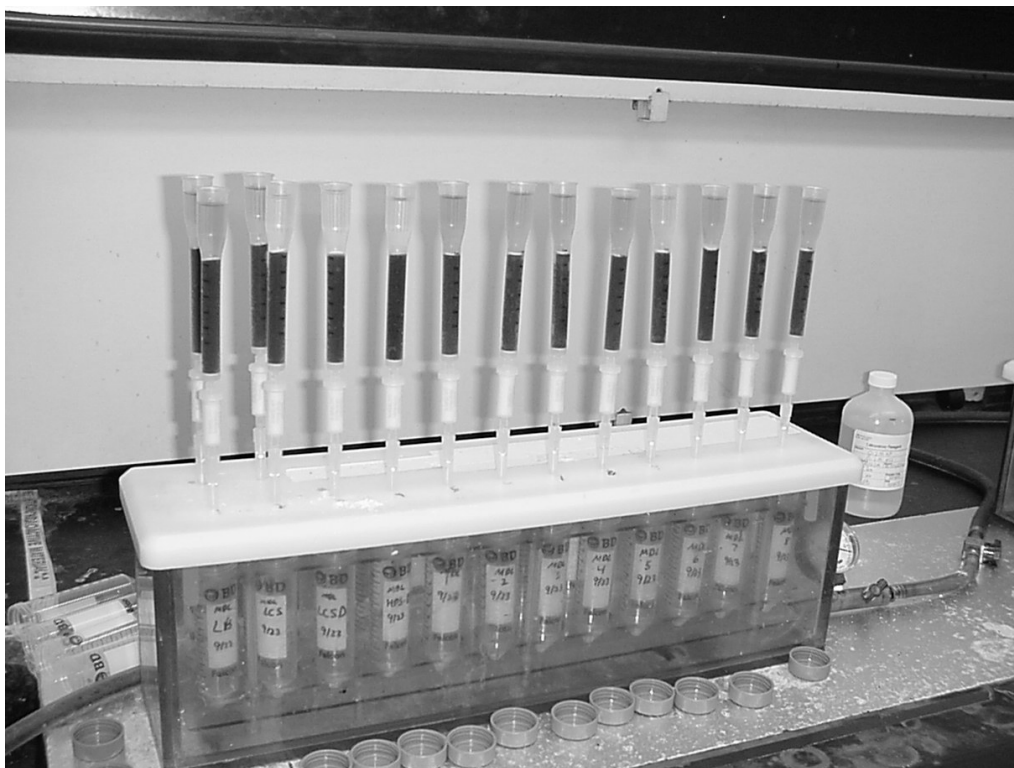
Figure 3 Vacuum Box System with Diphonix Resin and TEVA cartridges
