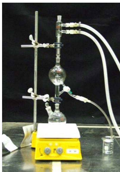
Figure 2-1. Apparatus for Sludge Boiling Evaluation
