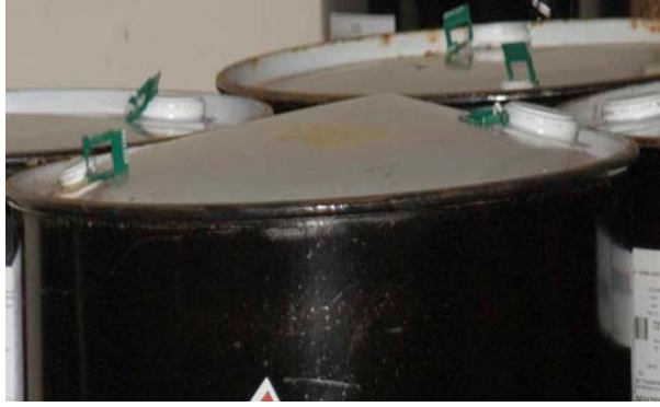
Figure 1. Bulged lid of stored 55 gallon wastewater.
