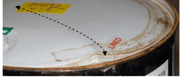
Figure 4. The drum lid crease is shown below dotted line. Drum Label reveals the United Nations uniform drum designation, 1A1/X1.8/300/05/USA.
