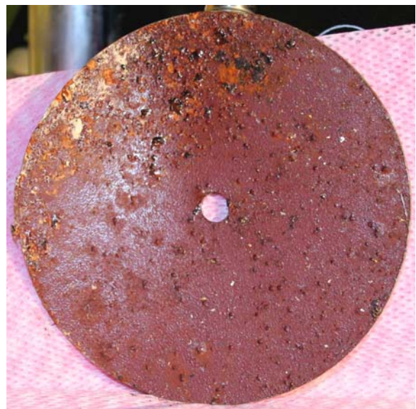
Figure 6. ID surface cut from bulged drum head revealing visible corrosion.
