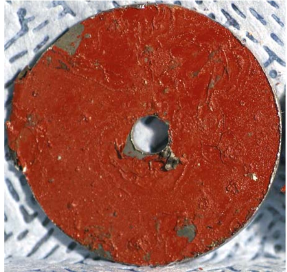
Figure 9. ID surface from non-bulged 1115 drum side-wall.
