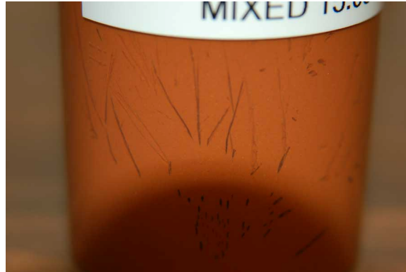
Figure 3-2 Crystals in the NoRCRA Insoluble Salt Simulant
