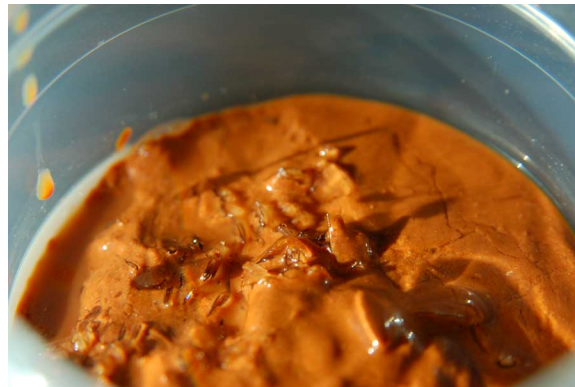
Figure 3-4 Sodium Carbonate Decahydrate Crystals in Insoluble Salt Simulant
