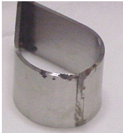
Figure 17. Stress corrosion cracking along the autogenous weld in coupon 304L – 20 from container 4a-2
