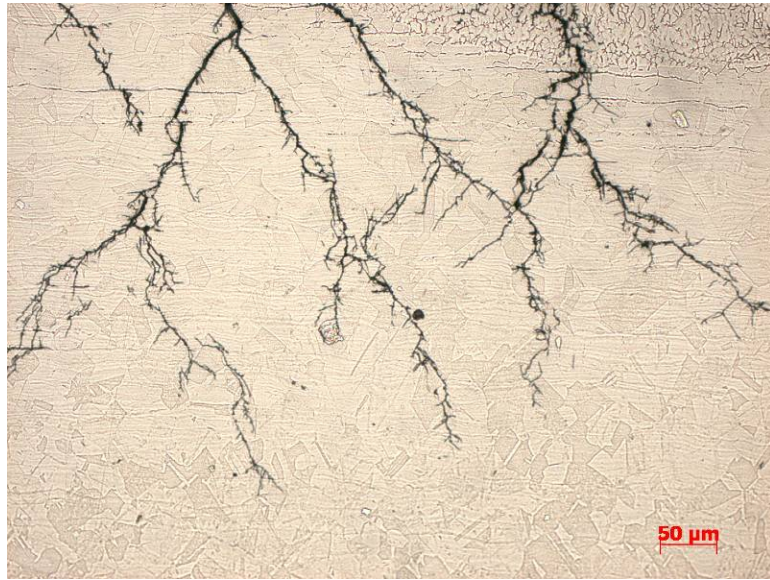
Figure 16. Optical micrograph showing transgranular nature of the cracking.
