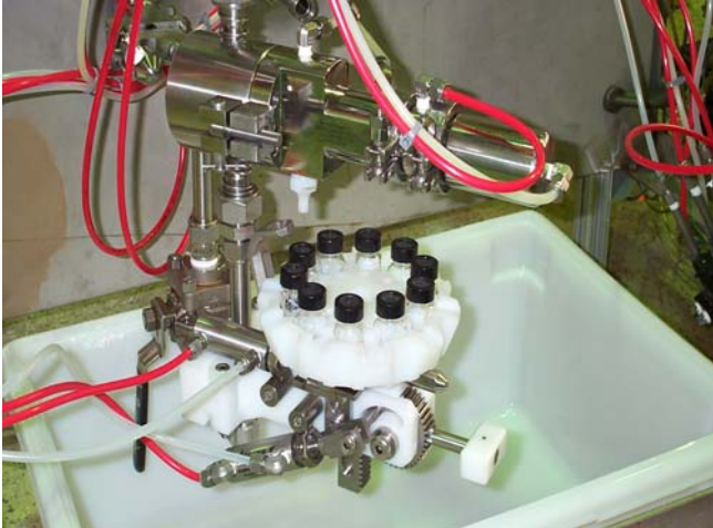
Fig. 7 Isolok rotary multi-sampler with ten sampling vials
