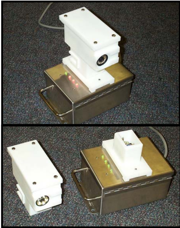
Fig. 9 Sample Cell Wireless Camera and Charger
