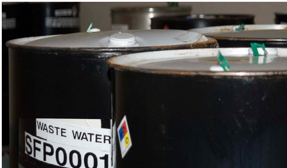
Figure 3. Close-up view of normal depressed lids on two adjacent drums compared with bulged drum lid to the left. Bulged drum number is SFP000117.
