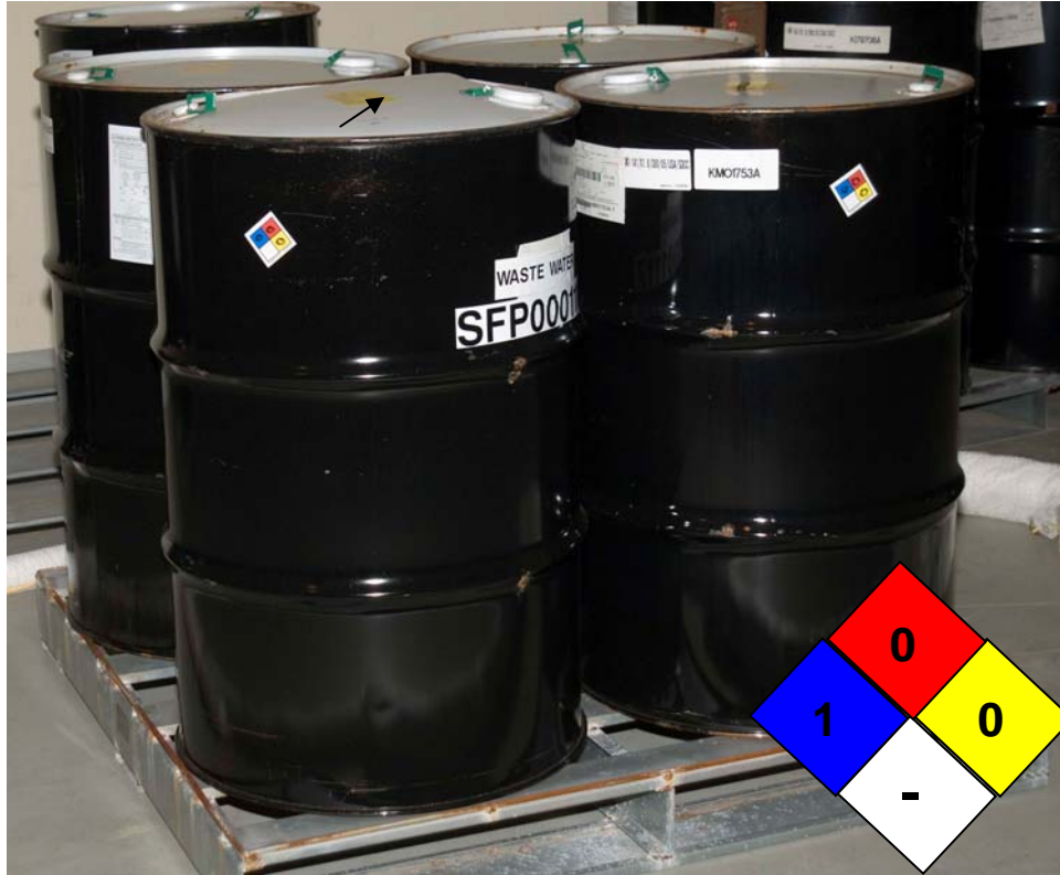
Figure 2. Bulged drum (A) on pallet along with three additional drums containing wastewater. The NFPA hazard label is reproduced in lower right corner.
