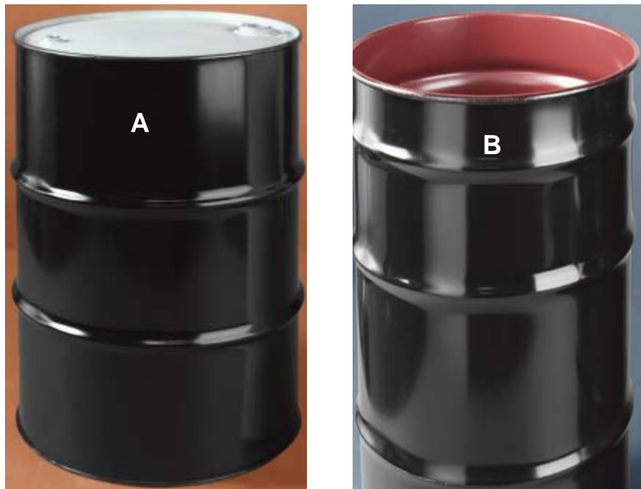
Figure 5. Exterior view of new 55 gallon carbon steel tight head drum (A) in left photo with red epoxy phenolic lined drum (B) shown in right photo (Vendor photographs). Note that the B drum has an extra rolled hoop near the top. SRS drums have two roll hoops as shown in A.
