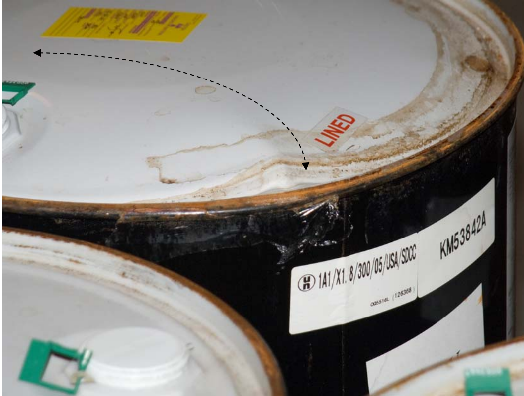
Figure 4. The drum lid crease is shown below dotted line. Drum Label reveals PO No. KM53842A” with the United Nations uniform drum designation “1A1/X1.8/300/05/USA/SDCC.” The designation “SDCC” identifies Skolnik Industries as the manufacturer.
