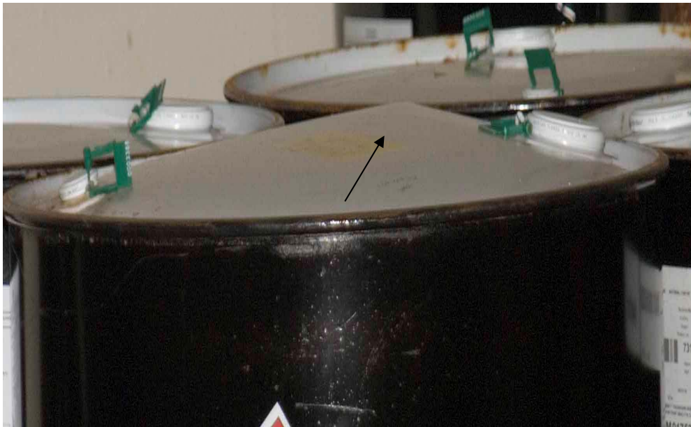
Figure 1. Bulged lid of 55 gallon wastewater drum stored in L-Area.
