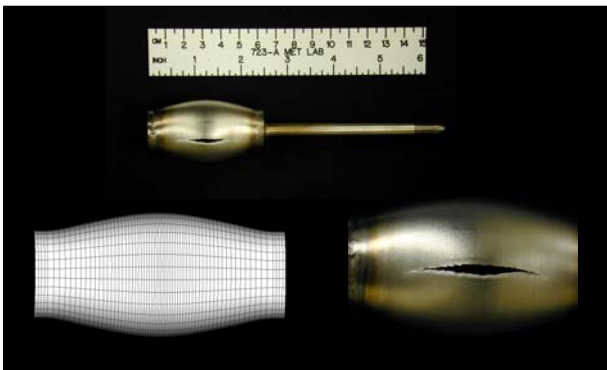
Figure 10. Burst Cylindrical Vessel and Finite-Element Model Showing Agreement Between Deformed Shapes (7).
