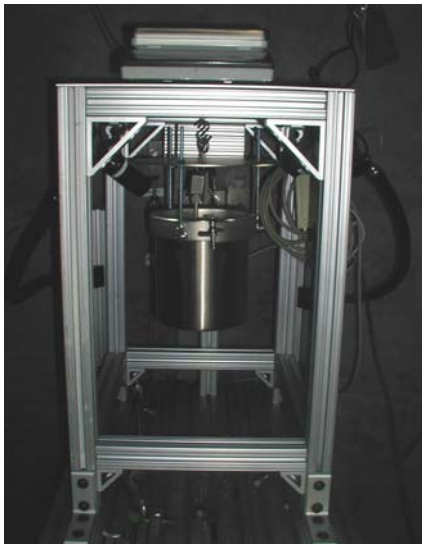
Figure 3. Set-up for Burst Testing in High Pressure Laboratory.
