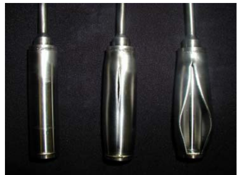
Figure 5. Burst Test Sample From Left to Right: New, Hydroburst, Deuterium Burst
