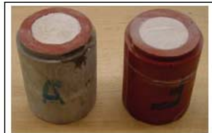
Figure 1. Saltstone potted in epoxy casts for permeability analysis. Grey is the aluminum based epoxy and the red is the ceramic based epoxy.
