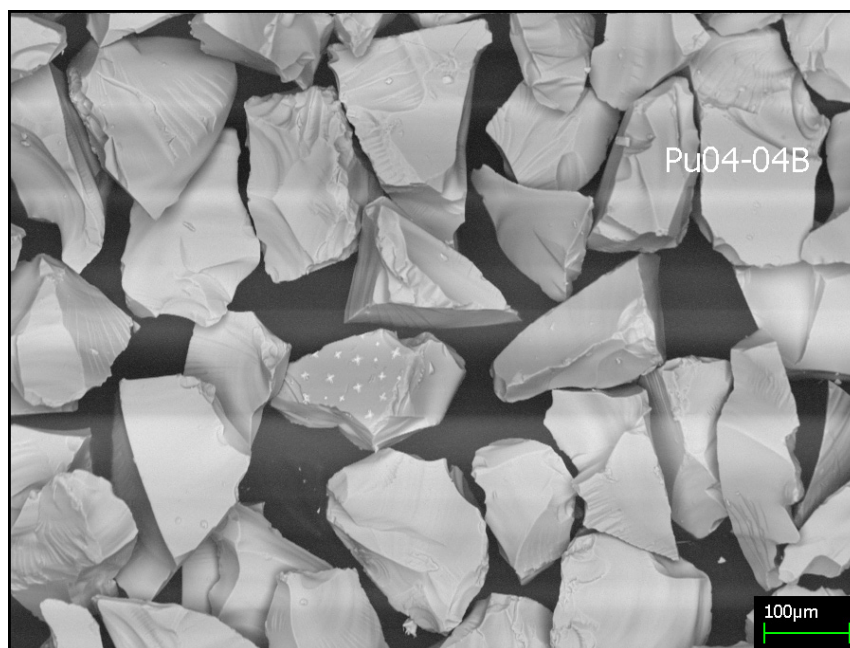
Figure 3. Higher magnification SEM micrograph of glass Pu04-04B, showing a small area of crystalline material.
