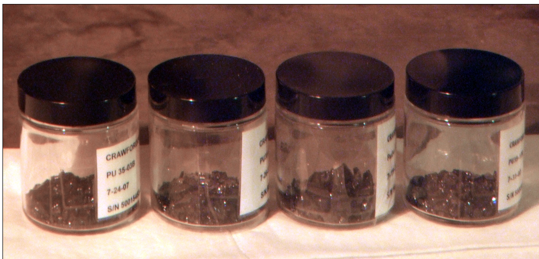
Figure 1. Photograph of the four glasses fabricated with \text{PuO}_2 in the SRNL shielded cells facility. The glasses are, from left to right, Pu35-03B, Pu35-06B, Pu04-04B and Pu35-17B.
