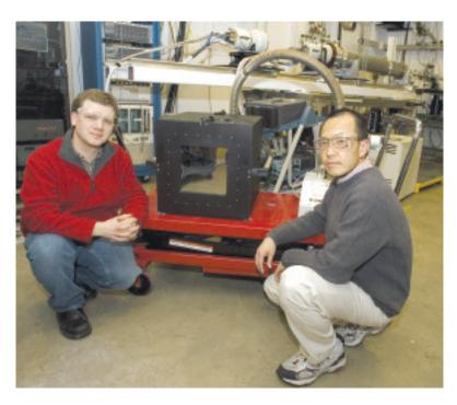
Tim Madden (left) and John Lee of the BTS Group, with the small-angle x-ray scattering detector in the 12-ID research station. The detector, which was designed and fabricated by BTS specifically for 12-ID, has four fiber-optic coupled CCDs, for a total active area of (170 mm)<sup>2</sup>.
