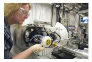
Kathy Kitts in the GSECARS research station, mounting one of the Genesis Probe samples (under the yellow plastic cover) prior to data taking.
