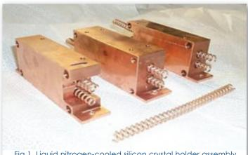
Fig.1. Liquid nitrogen-cooled silicon crystal holder assembly for the 20-ID-A monochromator.
