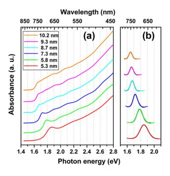
**Figure 4.** (a) Representative absorption spectra of CdTe quantum wires of various diameters in the range of 5.3-10.2 nm. (b) Lowest-energy excitonic peaks extracted by nonlinear least-squares fitting.
