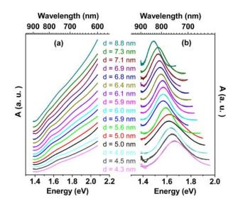
**Figure 2.** (a) Representative absorption spectra of InP wires; wire diameters (*d* values) are given in the key; and (b) Lowest-energy excitonic peaks extracted by nonlinear least-squares fitting and background subtraction (various colors), and the Gaussian fits to those peaks (gray). Wires synthesized under various conditions are included (see Table 1 in the Supporting Information); which in some cases produced separate quantum-wire specimens having the same diameters.
