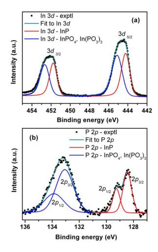
**Figure 9.** XPS from HF-photoetched InP wires (HF/InP = 52/1, etching time = 120 h under filtered xenon irradiation). (a) In3*d* core level; and (b) P2*p* core level. Binding energies and FWHM are listed in Table 4 in the Supporting Information.
