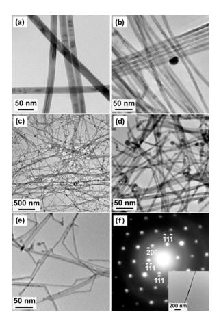
**Figure 1.** TEM images of InP wires (mean diameter  $\pm$  one standard deviation in the diameter distribution, expressed as a percentage of the mean diameter). (a) 19.0 nm  $\pm$  24.2%, (b and c) 11.2 nm  $\pm$  17.5%, (d) 6.9 nm  $\pm$  16.1%, (e) 5.6 nm  $\pm$  13.2%, and (f) electron-diffraction pattern in an [011] zone from the quantum wire shown. The observed reflections are indexed, demonstrating the [111] orientation of the wire.
