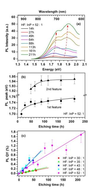
**Figure 5.** HF-photoetching of InP wires under a filtered xenon lamp ( $\lambda > 700$  nm). (a) PL spectra at different etching times with HF/InP = 52/1. The red dashed arrows are guides to the eye; (b) Etching-time dependence of PL-peak energy shift (HF/InP = 52/1). The black curves are guides to the eye; and (c) Effective PL quantum yield as a function of etching time at various HF/InP ratios. The lines are linear least-squares fits to guide the eye.
