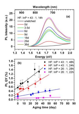
**Figure 8.** Photo-aging of HF-photoetched InP wires under room light. (a) PL spectra at different aging times after 14 h of photoetching with HF/InP = 43/1; and (b) Effective PL quantum yield as a function of aging time. The legend shows the HF/InP ratios and etching times. The lines are linear least-squares fits to guide the eye.
