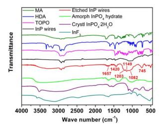
**Figure 10.** FTIR spectra for unetched (black) and HF-photoetched InP wires (red, HF/InP = 52/1, etching time = 88h under filtered xenon irradiation). The spectra for myristic acid (MA, olive), HDA (blue), TOPO (pink), amorphous InPO<sub>4</sub> hydrate (green), crystalline InPO<sub>4</sub>·2H<sub>2</sub>O (purple), and InF<sub>3</sub> (dark cyan) were added for comparison.
