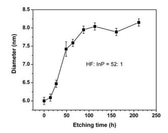
**Figure 7.** Plot of TEM wire diameter as a function of etching time (HF/InP = 52/1). The black curve is a guide to the eye. The error bars are the difference between the statistical mean diameters and the peaks of the Gaussian fits to the diameter distributions (see Supporting Information and Figure S13 for details).
