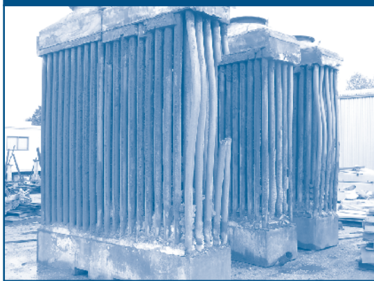
Figure 1. Example of a poorly maintained heat exchanger from an aluminum melting furnace
