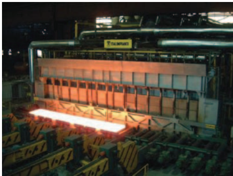
A walking beam furnace for metal reheating.
