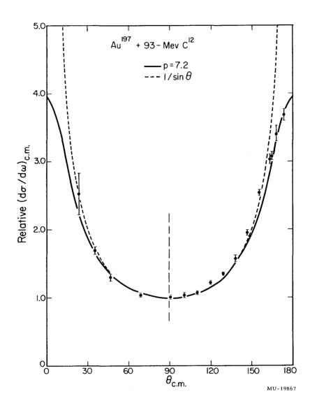
Fig. 6. Center-of-mass angular distribution of fragments from fission of Au<sup>197</sup> induced by 93.3-Mev C<sup>12</sup> ions. The solid curve represents Halpern and Strutinski's theoretical angular distribution with p=7.2 (see text).
