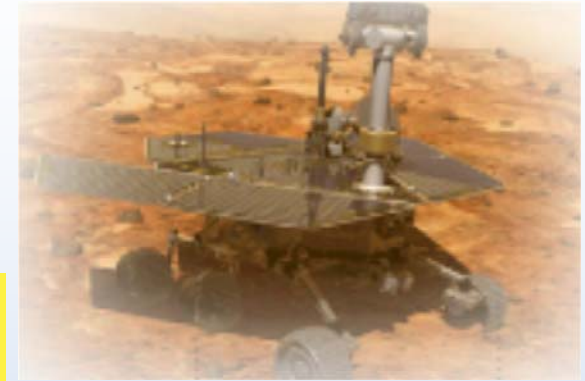
Mars Rover powered by multijunction cells
