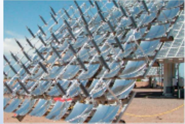
Microdishes can be passively cooled
