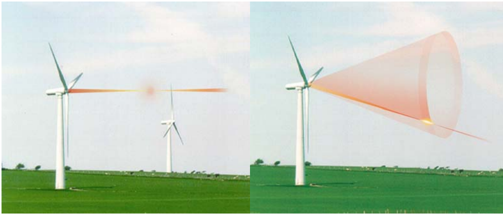
Figure 7: Wind turbine inflow measurements using hub-mounted LIDAR .
