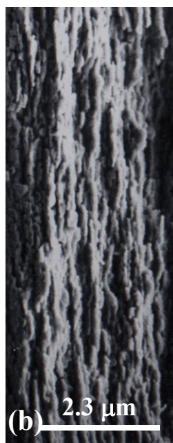
Higher resolution image of the LiOH corrosion layer
