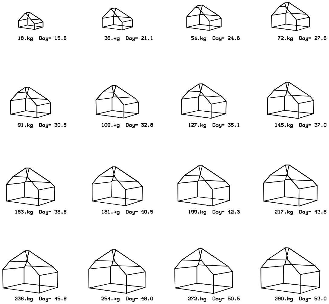
Figure 14. C-49 crystal shapes as a function of time (large anti-pyramid present on face 4, the back left face in this perspective, is not shown)
