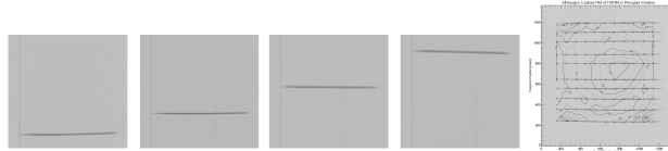
Fig. 5. Sequence of multiple temporal resolution images acquired with different trigger delays. These images are combined to derive the temporal resolution contour plot.
