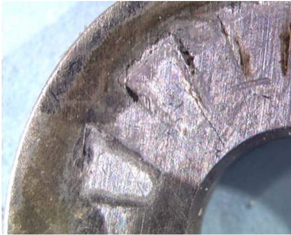
Figure 7 – Specimen JE1714 after CPP in Electrolyte 3, R = 0.01 at 90°C. Crevice corrosion and transpassivity are observed.
