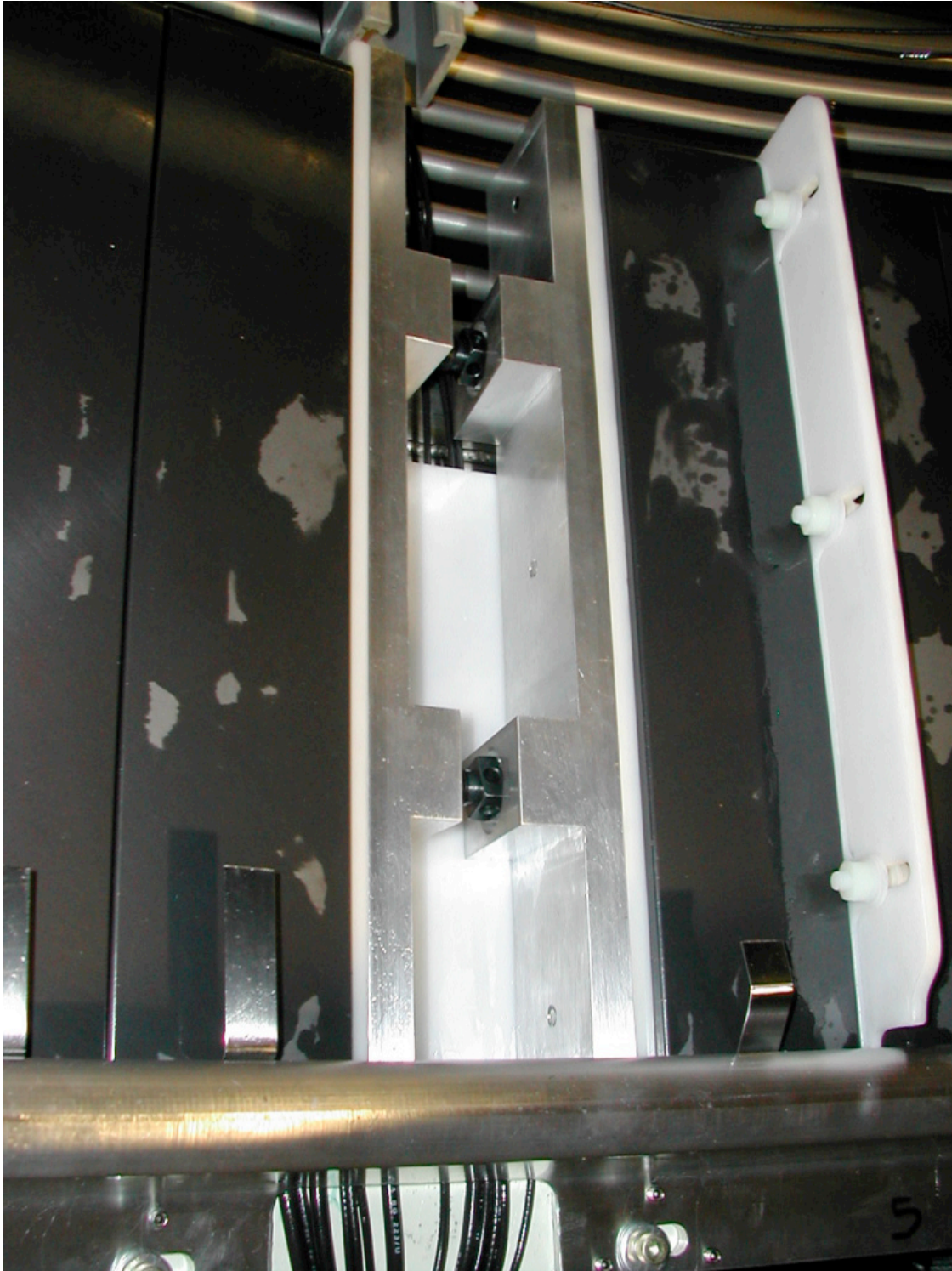
Figure 5.6 Loading plate at last space on west side. The double wedge spacer can be seen on the right side and the 16 RG223 cables can be seen behind the aluminum shelf at the bottom of the photo. The shims between each ferrite tile and the shelves are removed after assembly.
