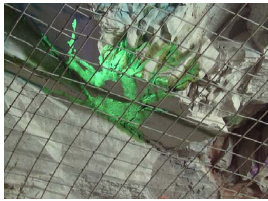
Figure 4-4. Water containing fluorescent dye seeps out of fractures intersecting the ceiling of an underground opening during an artificial infiltration experiment performed at Yucca Mountain.
