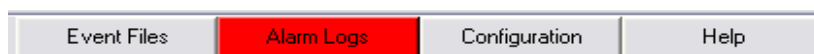
Figure 12: “Alarm Logs” Tab Highlighted in Red to Alert RTDMS User of New Alarm
