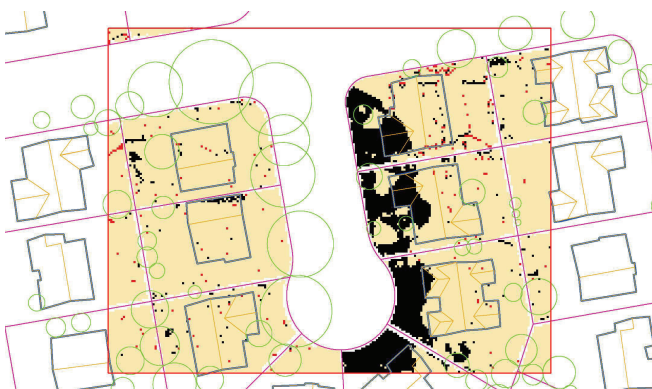
Fig. 6: Detail of extraparcels shadow raster (total shadow raster minus intraparcels shadow raster) on June 21 at 5P LST. Black cells are shaded; isolated black cells and all red cells are computational artifacts.
