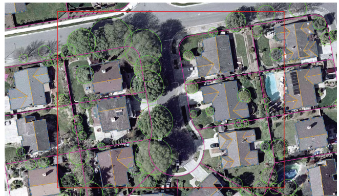
Fig. 2: Roof (blue), plane (gold), tree (green) and parcel (magenta) shapes overlaid on detail of orthophoto.
