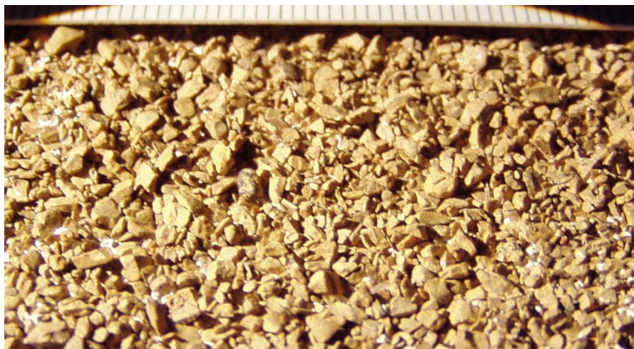
Fig. 1. Photographs of tested shingles with 2stdbf granules (see Table 1): (a) pilot plant shingle, (b) hand-made shingle with black paint as adhesive, and (c) hand-made shingle using white paint as adhesive. The ruler shows millimeters.
