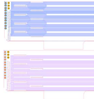
Figure 2. The connection end regions of the circuit board layer 1 (top) and layer 2 (bottom) showing the 8 blocks of conductor ‘loops’ of the odd and even probe layers. Loops 1-8 refer to loops shown from top to bottom.
