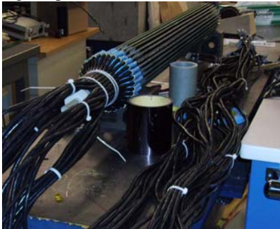
Figure 1. The fixed coil probe with 32 radially mounted circuit board probes.
