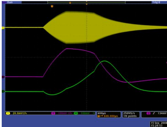
Figure 9: Vectorsum and IF signal for the Lorentz force detuned cavities
