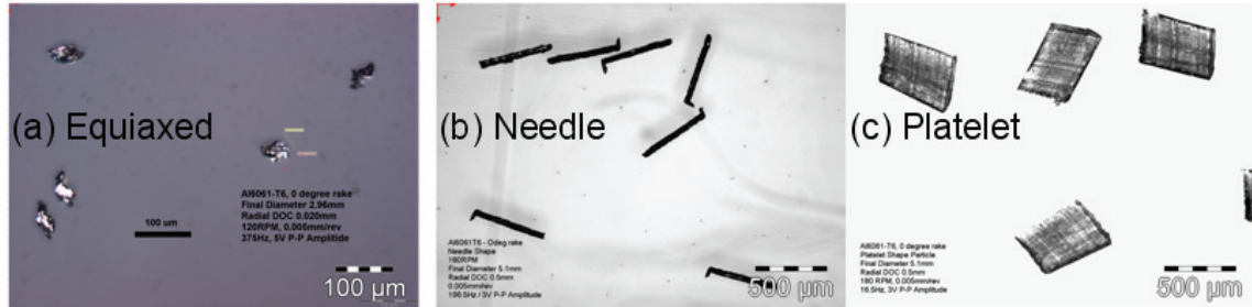
Figure 3-2 Optical Microscopy Images of Different Shape Particulates Created by MAM of Aluminum 6061-T6 Alloy (Machining and Modulation Parameters are Given in Table 3-2)
