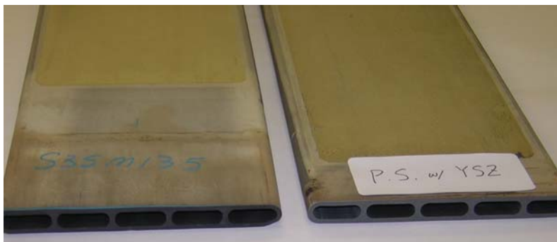
Figure 1-73. Comparison of H PD once-through cells without (left) and with (right) plasma-sprayed YSZ coatings
