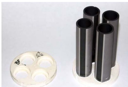
Figure 1-75. Pictures of spinel manifold testing coupons with surface plasma-sprayed with dense YSZ layer. The picture on the left is a bare sample without coating. The one on the right side was coated with YSZ and sealed with four cylindrical tube sections
