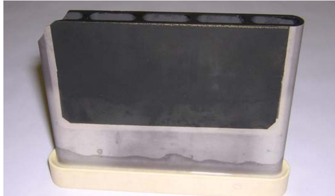
Figure 1-72. Picture of an AE HPD section sealed to a sense ZrO 2 cap using #57 seal
