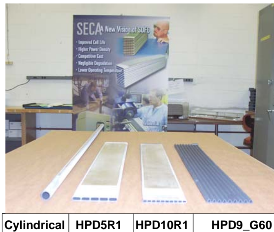
Figure 1-40. The types of tubes and cells currently available at Siemens Westinghouse
