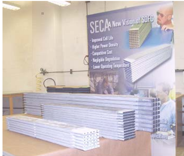
Figure 1-41. Different types and sizes of bundles currently fabricated at Siemens Westinghouse
