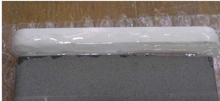
Figure 2-8. A “once-through” HPD cell sealed with a dense ZrO 2 cap using #82 glass seal
