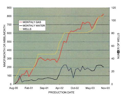
Figure 100: Summary of monthly gas and water production from Pod D wells. Note relatively low water production and very high gas production rates.
