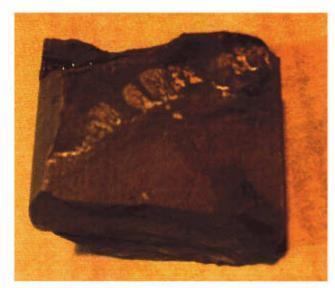
**Termination of an extension Fracture** Depth: 1261.1 ' Host Rock: siltstone
