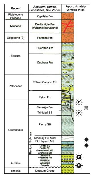
Figure 2: Geologic column of the Raton Basin area. Symbols to the right of the column indicate gas (white/open symbols) and oil (black/closed symbols) shows and/or production (modified after Dolly and Messier, 1977).
