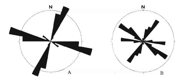
Figure 41: A) Rose diagram of fracture orientations within the sandstones, ring equals 20%, n = 33. B) Rose diagram of fracture orientations within the igneous sill, ring equals 20%, n = 49. There is a parallel relationship between many of the fractures within these two units of differing composition and age.
