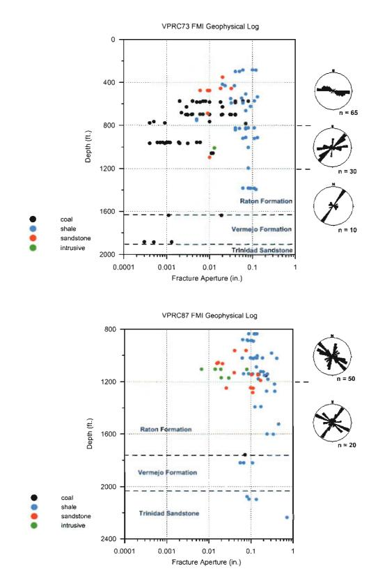
**Figure 60a:** Fracture hydraulic aperture estimated from the FMI logs for wells VPRC 73 and VPRC 87 versus depth. Lithology of fractures indicated by colored symbols. Rose diagrams of fracture strike are shown for different depth ranges to the right of the plot.
