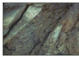
Close-up of 15 cm thick fault smear (knile for scale). Smear consists of amorphous clay with coaly inclusions, suggesting incorporation/injection along the fault prior to https://cation.
