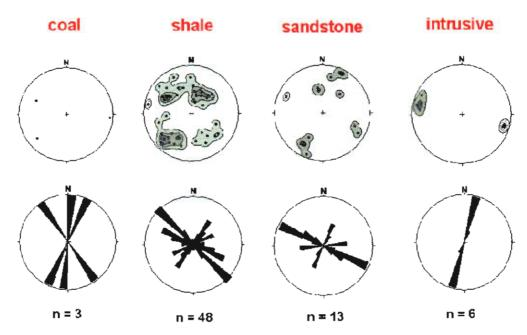
Figure 61a: Orientations of open fractures from FMI logs for wells VPRC 73 (above) and VPRC 87 (below), classified by lithology. Stereonet plots show lower hemisphere projections of fracture poles.
