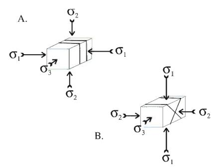
**Figure 56:** Block diagrams showing relations of stresses to fractures at two different depths. A)  $\sigma_1$  and  $\sigma_2$  are constrained only to lie in the fracture plane. B) The stress system shown is unique for conjugate normal fractures.
