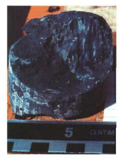
Figure 18. Compaction fracture in fine-grained silty mudstone of the Raton Formation.
