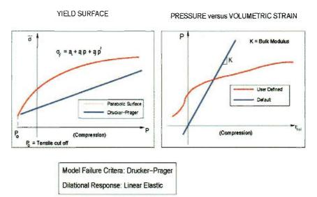
Figure 75: Soil and foams material model.
