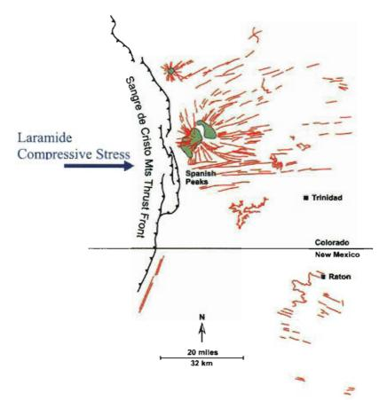
Figure 10: Map of larger scale intrusions within the Raton Basin. Due to the map scale numerous small dikes and sills are not shown. Volcanic intrusions are paleostress indicators.
