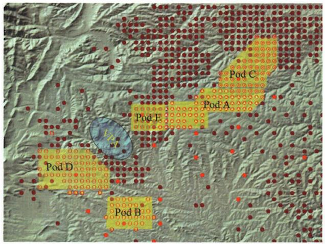
**Figure 94**: Subset of Figure 1, showing arrangement of CBM wells operated by El Paso Raton LLC in the New Mexico portion of the Raton Basin. Note position of well "Pods" relative to the Vermejo Park Anticline (VPA).
