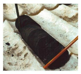
**Perpendicular Extension Fractures** Depth: 1192' Host Rock: Shale
