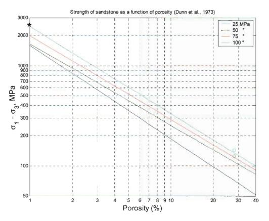
**Figure 1:** Maximum stress difference at failure for various sandstones plotted against porosity. Lines for the four different confining pressures indicated in the upper right. Circles are Sandia data for Castlegate sandstone of 28% porosity. The confining pressures for Castlegate are indicated by the same color code as the lines: cyan is 100 MPa, and (light) green is 50 MPa.
