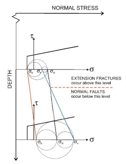
**Figure 57:** States of stress in relation to the failure condition at the two different depths referred to in the text.
