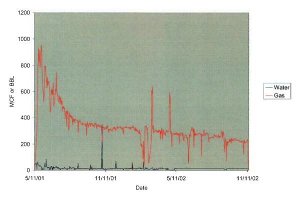
**Figure 105:** An example of high gas, very low water production typical of many wells in Pod D. Production behavior such as this would be more likely anticipated in a conventional gas reservoir rather than a coalbed methane field.
