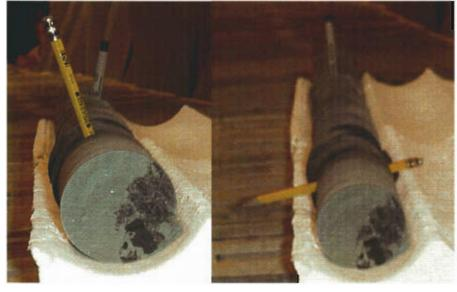
a.) Fracture Dip Directions of two fractures with a strike intersection of  $30^{\circ}$  are shown with a pen and pencil.
