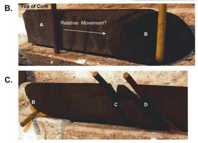
**C:** Continuation of the core seen in Figure B. Fractures C and D strike normal to Fracture C.
