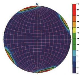
**Figure 18:** Pole to plane stereonet of fracture orientations within the Dakota Sandstone near mile markers 374 and 375 on Hwy 160; n=198. These data show the majority of fractures have near vertical dips and conjugate strikes.
