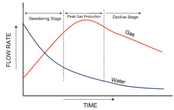
**Figure 93:** Idealized production behavior of a typical coalbed methane well. Pressure in the coal seam is reduced by pumping off formation water. Methane production increases with decreasing formation pressure.
