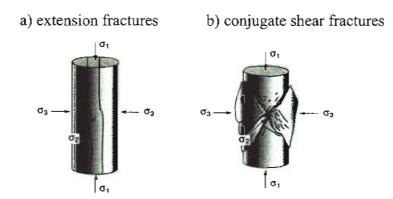
Figure 13: Extension and conjugate shear fractures as observed and created in laboratory compression tests ( $\sigma_1$  – maximum principal stress;  $\sigma_2$  – intermediate principal stress;  $\sigma_3$  – minimum principal stress) (modified from Weijermars, 1997).
