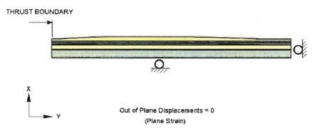
Figure 73: Model boundary conditions.
