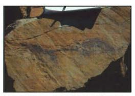
Fault surface where it cuts across sandstone (clip-board with pencil for scale). Lowrallel finantions suggest some inclusation of the sand but fack of gouge and sinckensides indicates it was not significant.
