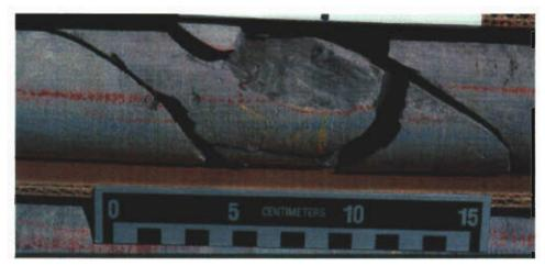
Figure 17. Shear fractures in muddy siltstone of the Raton Formation. Note alignment of slickensides on the outward-facing fracture with the dip direction of the other two fractures.
