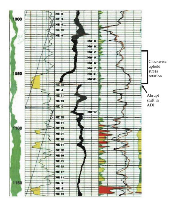
**Figure 65:** An example of the irregular uphole stress rotation typical within upper sections of the VPRC 87 and 73 holes. An abrupt shift at 1060 ft correlates to a fractured interval in the FMI log (Figure 66).
