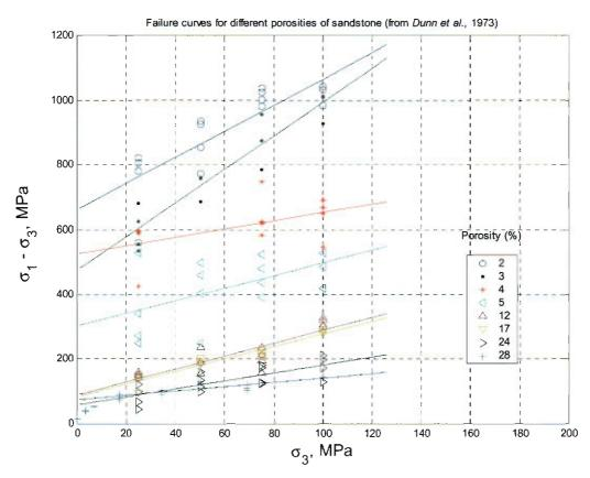
**Figure 2:** Strength versus confining pressure for sandstones of differing porosities. The 28percent-porosity rock is from *Olsson* (unpublished, and 1999) for Castlegate sandstone.
