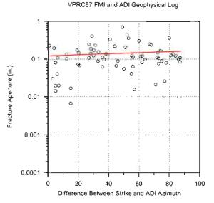
**Figure 62:** Fracture hydraulic aperture estimated from the FMI logs for wells VPRC 73 (upper) and VPRC 87 (lower) versus the angle between fracture strike and the local azimuth of the maximum horizontal compressive stress from ADI logs. The linear regression is shown as the red line in both plots.
