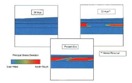
Figure 82: Maximum principal stress orientation.
