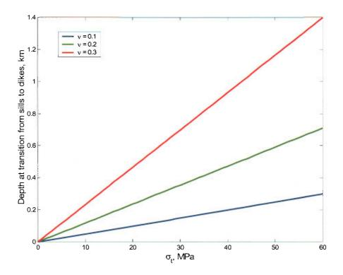
Figure 68: Depth below which dikes predominate and above which sills predominate plotted against tectonic stress for several values of  $\nu$ . Density  $\rho$  was taken to be 2300 kg m<sup>-3</sup>.
