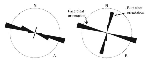
**Figure 34:** A) Rose diagram of fracture orientations in Vermejo sandstones on frontage road 2 miles south of Trinidad, CO. Ring equals 40%, n = 55. B) Rose Diagram of cleat orientations in Vermejo coals on frontage road 2 miles south Trinidad, CO. Ring equals 40%, n = 49.
