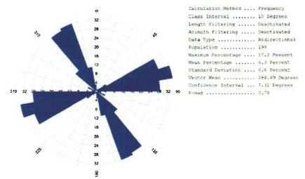
Figure 17: Rose diagram of fractures in the Dakota Sandstone near mileposts 374 and 375 on highway 160; n = 198.
