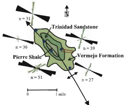
**Figure 46:** West-northwest oriented fractures are highlighted in black and are interpreted to predate fractures related to intrusion of Morley Dome. Red lines in the southeastern quadrant of the dome are igneous dikes. Gray cross fractures with variable strikes are probably related to the formation of the anticline.
