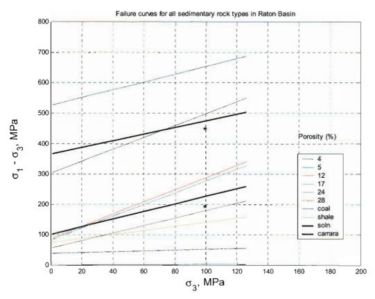
**Figure 5:** Failure curves for all major sedimentary rocks found in the Raton basin. All limestones fall between the two heavy black lines. The individual data points have been omitted for clarity. The two asterisks are for data from *Hugman and Friedman* (1979).
