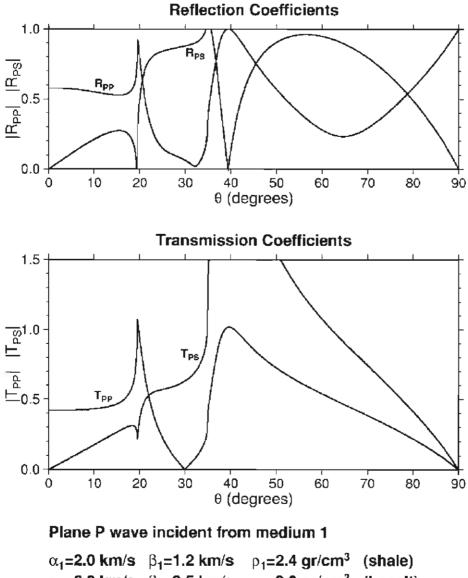
$\begin{array}{ll} \alpha_1 = & 2.0 \ \text{km/s} & \beta_1 = & 1.2 \ \text{km/s} & \rho_1 = & 2.4 \ \text{gr/cm^3} & (\text{shale}) \\ \alpha_2 = & 6.0 \ \text{km/s} & \beta_2 = & 3.5 \ \text{km/s} & \rho_2 = & 3.0 \ \text{gr/cm^3} & (\text{basalt}) \\ & \text{critical angles:} & \theta_{\text{crit}} = & 19.5^\circ, \ 34.9^\circ \end{array}$
