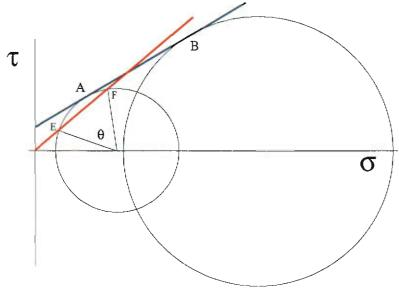
Figure 6: Mohr plot for intact (blue,  $tan\phi = 0.6$ ) and friction on interface (red,  $\mu = 0.85$ ). Angular range over which slip occurs before intact failure given by  $\theta$ .
