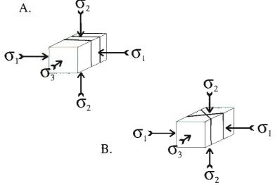
**Figure 54:** A) Stress orientations *consistent* with extension fractures. B) Stress orientations *required* for strike-slip shear fractures. The orientations for both systems of fractures are identical.
