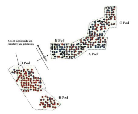
Figure 15: Pie chart map showing relative amounts of water (blue) and gas (red) produced on a daily averaged basis. The best gas producers of the lease are near where we are standing.
