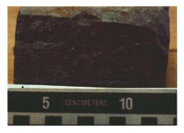
Figure 14. Plumose structure on an extension-fracture surface in core from the Raton Formation.
