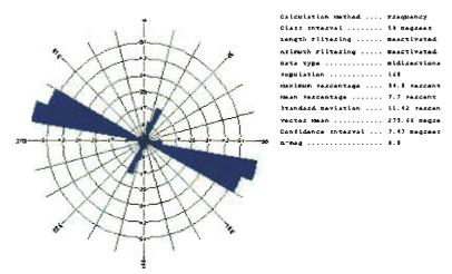
**Figure 24:** Rose diagram of fractures within the Niobrara Limestone between milepost 365 and 366 on highway 160 (n=168). Note that the major fracture set strikes NW-SE and actually would bisect the acute angle of the fractures observed within the Dakota Sandstone (Figure 25).
