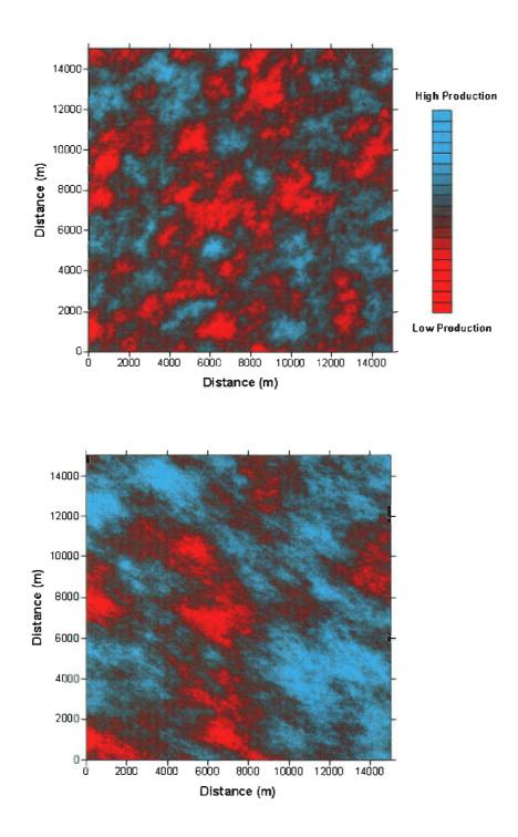
**Figure 111:** Unconditional simulations of relative average daily gas production, based on differing anisotropic values of variogram range, for Area 1 (upper) and Area 2 (lower) in the Raton Basin.
