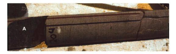
Parallel Extension Fractures Depth: 1204' Host Rock: Sandstone Fracture A may have dead oil stain on the surface. The fracture spacing is 0.05.
