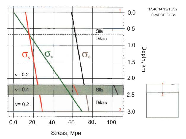
Figure 71: Two-dimensional, elastic model. The host rock is uniform sedimentary rock with  $\nu = 0.2$  containing a single layer of coal (gray) with  $\nu = 0.4$ . The vertical line indicated by the red numerals 1 and 2, is the line along which the stresses were plotted.
