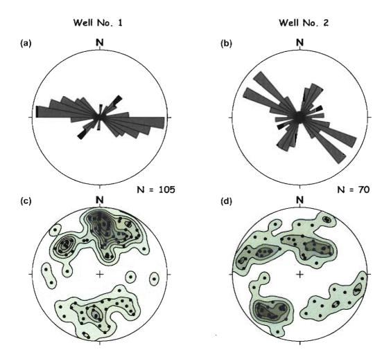
Figure 10. Orientations of open and partially open fractures as inferred from FMI logs from two holes in the southernmost Colorado portion of the Raton Basin. (a) and (b) Rose diagrams of fracture strikes; (c) and (d) lower-hemisphere stereonet diagrams for the same fracture populations shown in the rose diagrams immediately above showing poles to the fracture planes.
