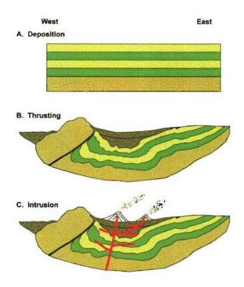
**Figure 11:** Simplified tectonic and depositional sequence of the Raton Basin. A) Initial deposition of sediments. B) Uplift and eastward thrusting of the Sangre de Cristo Mountains forms the basin. Syntectonic deposition also occurred within the basin at this time. C) Intrusion of magma into this geologic system formed laccoliths, stocks, dikes, and sills.
