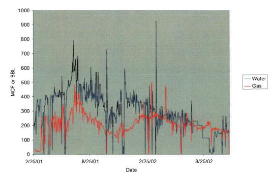
**Figure 103:** Gas and water production curves from a single well in Pod A. Contrast this production behavior with than in Figure 12. There is no well defined water decline, gas incline curve. Instead, peaks on water production are typically followed soon after by a peak in gas production.
