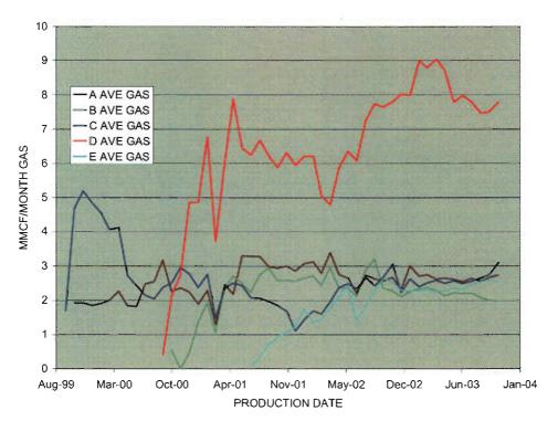
**Figure 96:** Average monthly gas production per well. Most wells in Pods A, B, C, and E are currently producing an average of 2.5 million cubic feet of gas per month. In contrast, the average production from wells in Pod D is three times greater.
