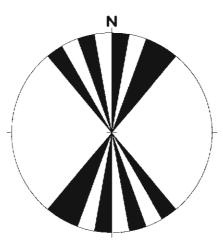
Figure 27: Rose diagram of faults within the Niobrara Limestone south of Springer, NM. Ring equals 20%, n = 5. Note the partial radial pattern and that this pattern bisects the obtuse angle of the fractures shown in Figure 26.
