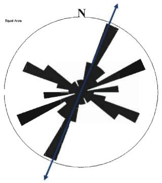
**Figure 22:** Rose diagram of fracture strikes from the Dakota Sandstone Wall (Figure 21) on the Vermejo Park Ranch (n=81). Fracture orientations are rotated back to horizontal. Strike of the folded "Wall" of Dakota Sandstone is shown as the blue arrow.
