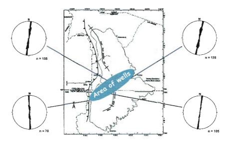
Figure 11. Rose diagrams showing consistency in orientation of present-day maximum horizontal stress in the central Raton Basin, as determined from DSI logging tool data. Precise locations obscured to protect proprietary data.
