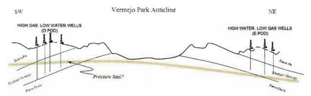
**Figure 106:** Conceptual cross section of Vermejo Park anticline illustrating one hypothesis for the differing gas to water ratios on either side of the structure. Production from Pod D southwest of the anticline may be from a basin-centered gas accumulation, which is isolated from meteoric waters by a capillary seal. Evidence includes low water production, high values of dissolved solids in the produced water, and increased water production at shallower depths.
