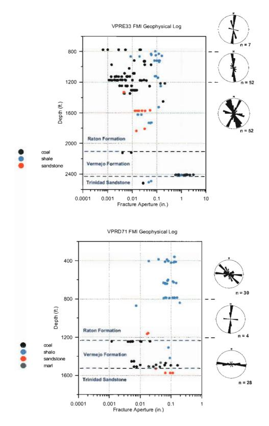
**Figure 60b:** Fracture hydraulic aperture estimated from the FMI logs for wells VPRE 33 and VPRD 71 versus depth. Lithology of fractures indicated by colored symbols. Rose diagrams of fracture strike are shown for different depth ranges to the right of the plot.
