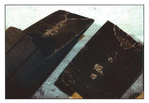
Extension Fracture (This fracture is the middle fracture in the photo shown above.)
