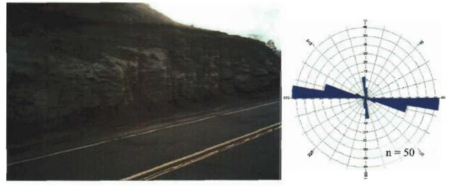
**Figure 32:** A) Uniform set of fractures within fluvial sandstones of the Vermejo Formation on Hwy 555 west of Raton, NM. B) Rose diagram illustrating fracture orientations at this site.
