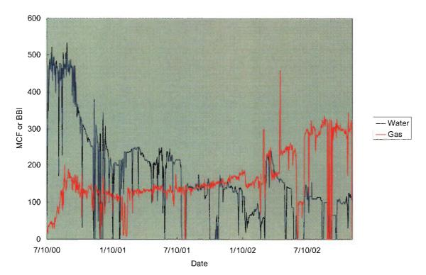
**Figure 102:** Example of gas and water production curves for a single well in Pod A. Compare with the idealized CBM production behavior in Figure 93. Wells of this type exhibit high initial water production and little gas production. Withdrawal of water from the formation decreases hydrostatic pressure and induces methane gas to desorb from the coal matrix. As formation pressure is reduced further, more gas desorbs from the coal, resulting in a gas incline curve.
