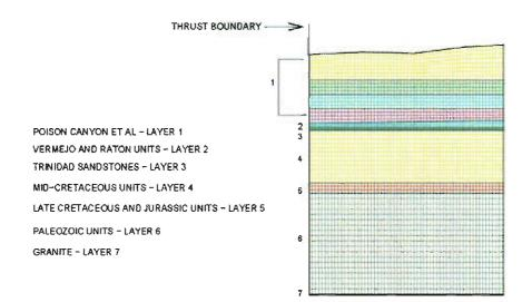
Figure 74: Mesh detail left-hand side of model.
