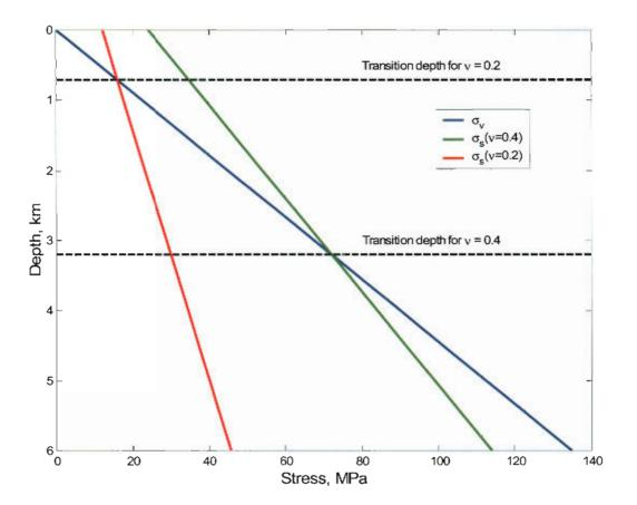
Figure 70: Vertical stress  $\sigma_v$  and  $\sigma_s$  plotted against depth for v=0.2, typical of sedimentary rocks, and v=0.4, representative of coal. The depth where  $\sigma_v$  exceeds  $\sigma_s$  is the transition depth from sills to dikes. This transition occurs at 0.72 km (2362 ft) for v=0.2. For v=0.4, the transition occurs at 3.21 km (10,531 ft).
