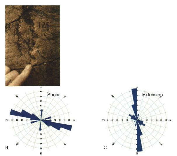
Figure 10: A) Steps instead of plumose structures on fracture surfaces indicate an origin in shear rather than extension. Shear indicators were found in the Raton Conglomerate in many locations around the Vermejo Park Ranch. Rose diagrams show difference in dominant orientation for shear fractures (B) versus extension fractures (C).
