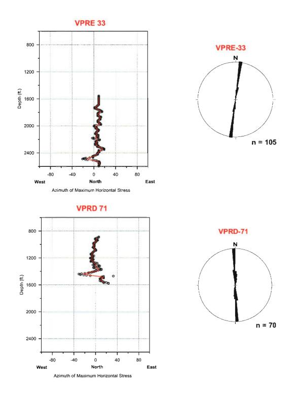
**Figure 64b:** Azimuth of the maximum horizontal compressive stress from the ADI logs from wells VPRE 33 and VPRD 71 versus depth. The red line shows the running average (over a 50 ft. window) of the azimuth of maximum horizontal stress. The rose diagrams to the right plot the corresponding values of the running average of the azimuth.
