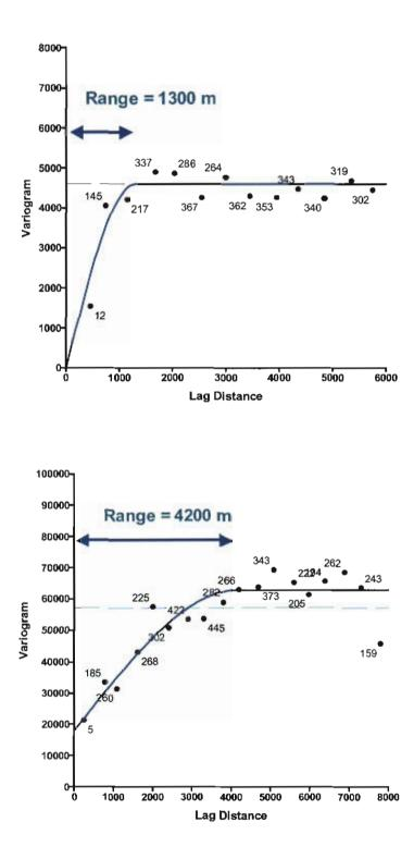
Figure 109: Omnidirectional variograms of average daily gas production in El Paso Production wells for Area 1 (above) and Area 2 (below) in the Raton Basin.
