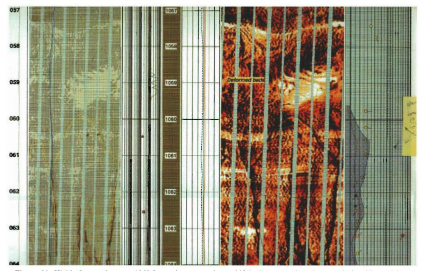
Figure 66: Highly fractured zone at 1060 ft correlates to an abrupt shift in the stress orientation on ADI log (Figure 65).
