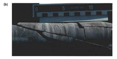
Figure 13. Near-vertical (approximately parallel to core axis) extension fractures in sandstones of the Raton Formation in core. Stratigraphic top is to the left. (a) Typical expression; (b) example of parallel fracturing.
