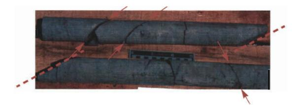
Figure 15. Reconstruction of in-situ core configuration for a reconstructed four (4) feet of core demonstrating the conjugate nature of a fracture set (solid arrows) in siltstone of the Raton Formation. The dashed lines indicate matched halves of the same fracture plane; Stratigraphic top is to the left and the core reads like a book from left to right and from top to bottom; scale is in centimeters.
