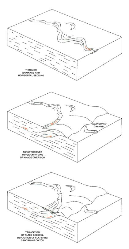
Figure 22: Suggested model to explain pre-lithification tilting and backthrusting of strata, with flat-lying fluvial strata in erosional contact above, at Ludlow and Cokedale sites.
