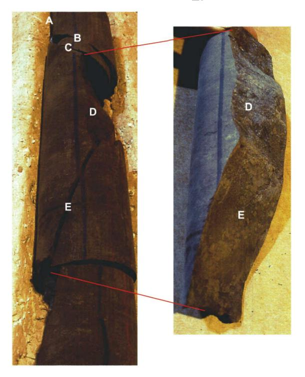
Fracture E is a vertical fracture that intersects Fracture D. The strikes of the two fractures intersect at a  $0^{\circ}$  to a  $30^{\circ}$  angle. The surface of the fracture is smooth and has patches of slickencryst.
