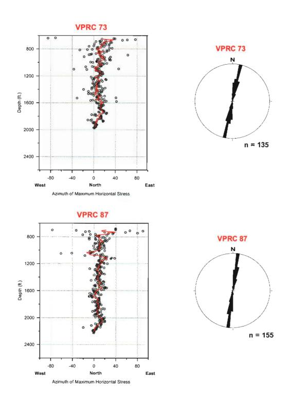
**Figure 64a:** Azimuth of the maximum horizontal compressive stress from the ADI logs from wells VPRC 73 and VPRC 87 versus depth. The red line shows the running average (over a 50 ft. window) of the azimuth of maximum horizontal stress. The rose diagrams to the right plot the corresponding values of the running average of the azimuth.
