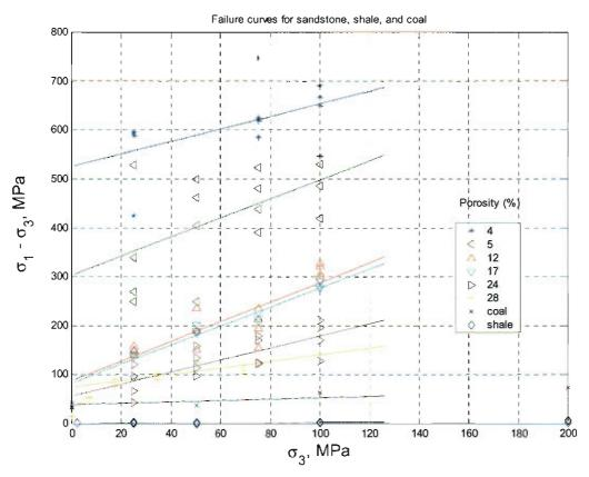
**Figure 4:** Strength map for clastic rocks and coal that may be typical of the Raton basin. Same as Figure 2 with the addition of curves for Pierre shale and sub-bituminous coal from Wyoming. Note that shale has a very low  $\sigma_0$  and vanishingly small (B-1). See Table 1.
