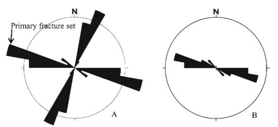
Figure 37: A) Rose diagram of primary throughgoing and secondary fracture orientations within Raton Fm sandstones near milepost 50 on Highway 12, n = 33. B) Rose diagram of the primary (oldest throughgoing) fracture set within Raton Formation sandstones on Hwy 12 near the intersection with county road 21.6, n=38.
