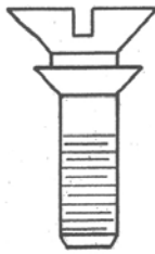
FOR DOUBLE COUNTER-SUNK HOLES
