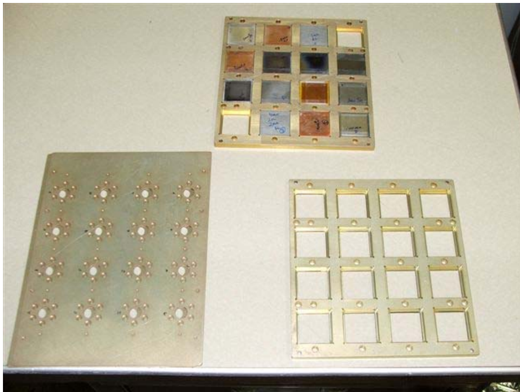
Figure 5 DAS with Filters Installed
