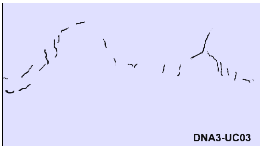
Figure 10. Unwrapped images of the induced fracture traces for frozen soil specimens subjected to unconfined uniaxial compressive stresses.
