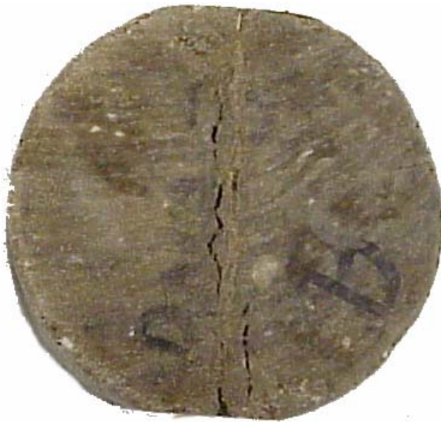
Figure 6. Typical displacement vs. load plot for fused frozen soil specimen with sol interface material. Induced tensile fractures independent from the fused interface are shown on the specimen.
