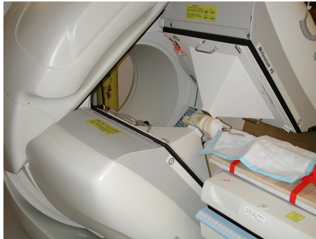
Figure 1. Pinhole SPECT scanner used for the dynamic cardiac data acquisition in a rat.
