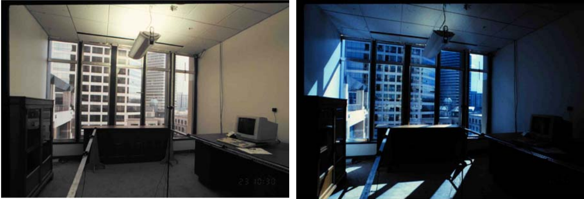
Figure 4 Initial testing of electrochromic glazings in GSA office building in Oakland CA.; left: glazing is clear under dark overcast conditions; right: glazing in lowest transmittance state with direct sun (Lee, et al. 2003).
