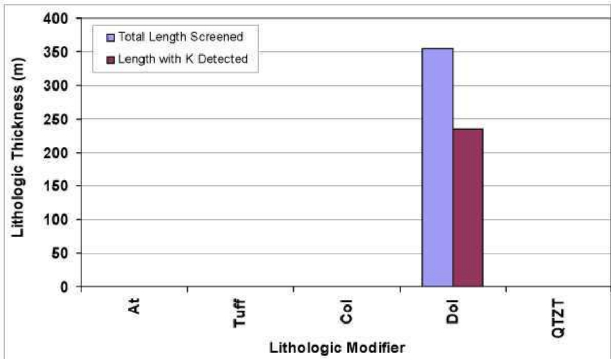
Figure 203. Lithologic modifiers adjacent to well screen and detectable hydraulic conductivity at well ER-6-1#2.
