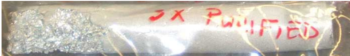
Fig. 4. Zinc sample, after 3 stages of purification.
