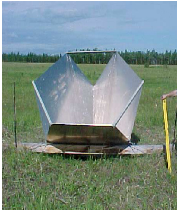
Figure 26. A 'trimmed' trihedral corner reflector for orbital SAR calibration. (courtesy of Wade Albright, Calibration Engineer, Alaska Satellite Facility)
