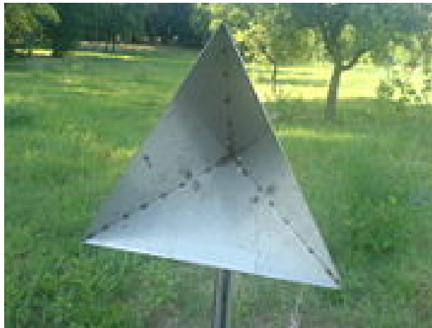
Figure 17. Trihedral reflector mounted on a pole. Note downward tilt of corner.
