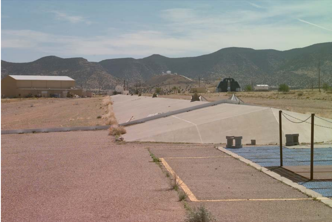
Figure 21. Sandia National Laboratories inverted "Vee" outdoor RCS test range. The stationary radar instrument is at the far end of the Vee. The device under test was mounted on a pedestal to the right of the camera. Currently the test range is used principally as a base for reflector placement for airborne tests. Note trihedral reflector array placed along peak of the Vee.
