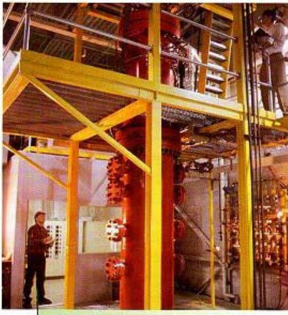
Figure 3. IPST's LEFR (top) shown with furnace open. Total height is 11 feet. Lower left is IPST's PEFR. Lower right is a CAD drawing of the PEFR. Total height is 35 feet.
