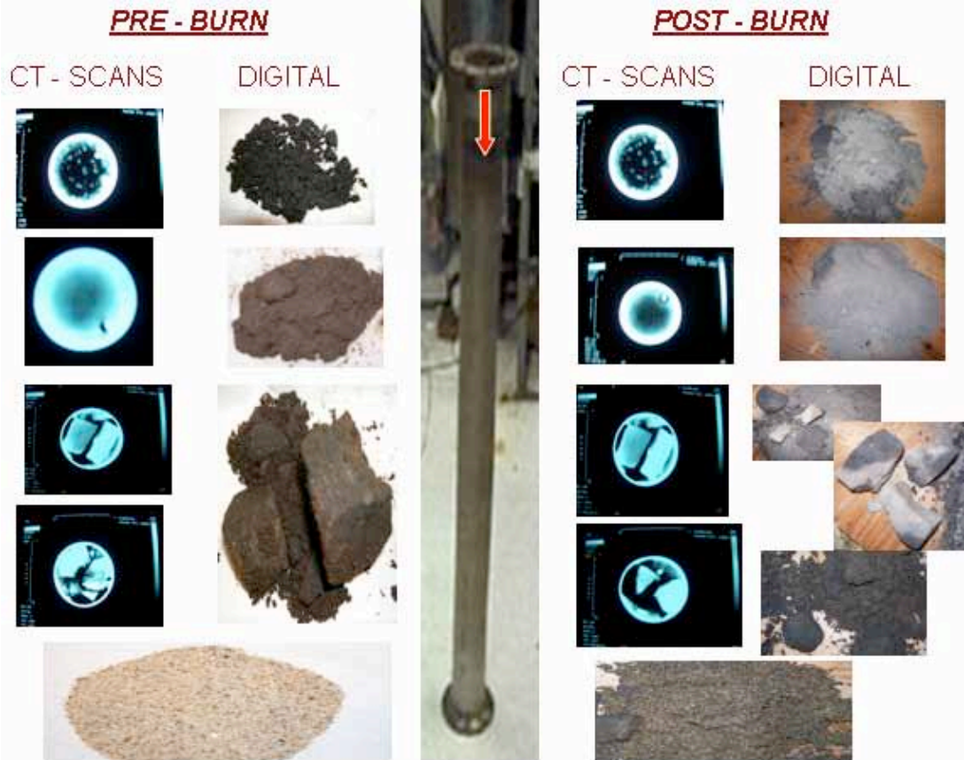
Figure 6.21. CT scans and digital images of pre and post-burn small-scale heterogeneous pack; experiment 9.
