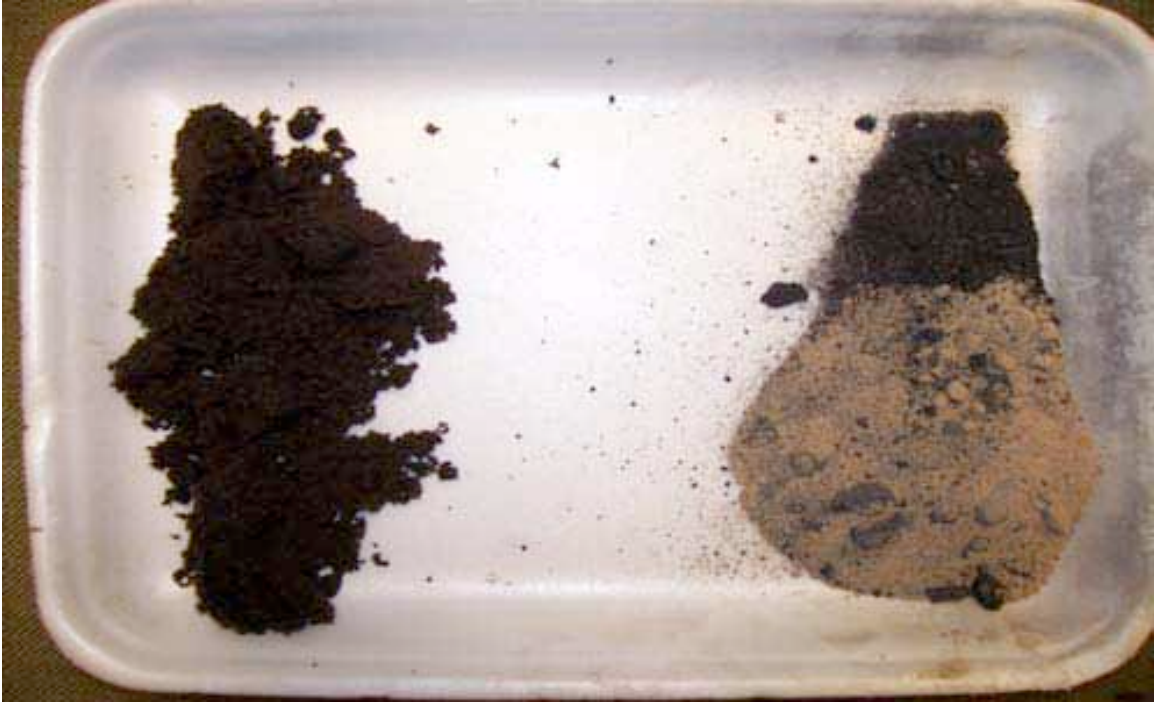
Figure 6. 13. Left - Crushed reservoir material before experiment at 50psig. Right - Residue after experiment at 50psig supply pressure. Note some coke-type particles in the residue.
