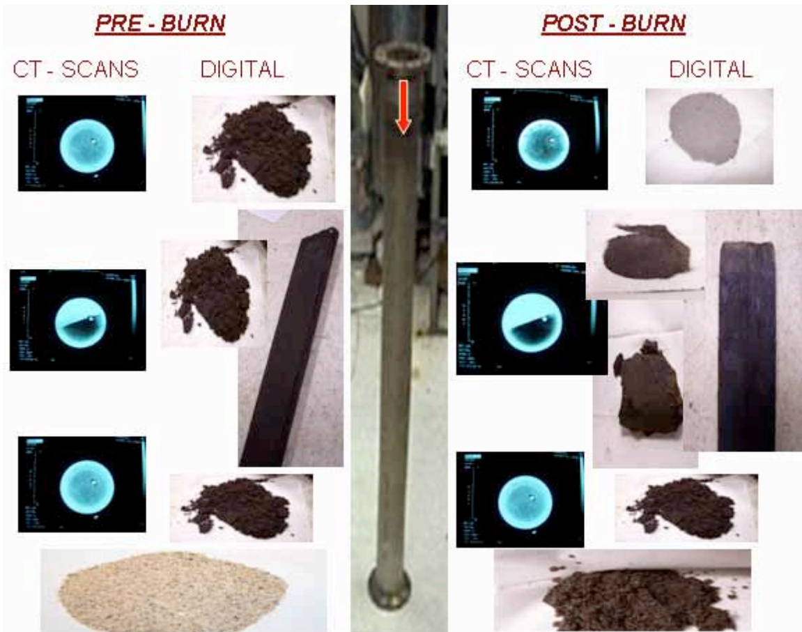
Figure 6.25. CT scans and digital images of pre and post-burn large-scale heterogeneous pack, experiment #10.
