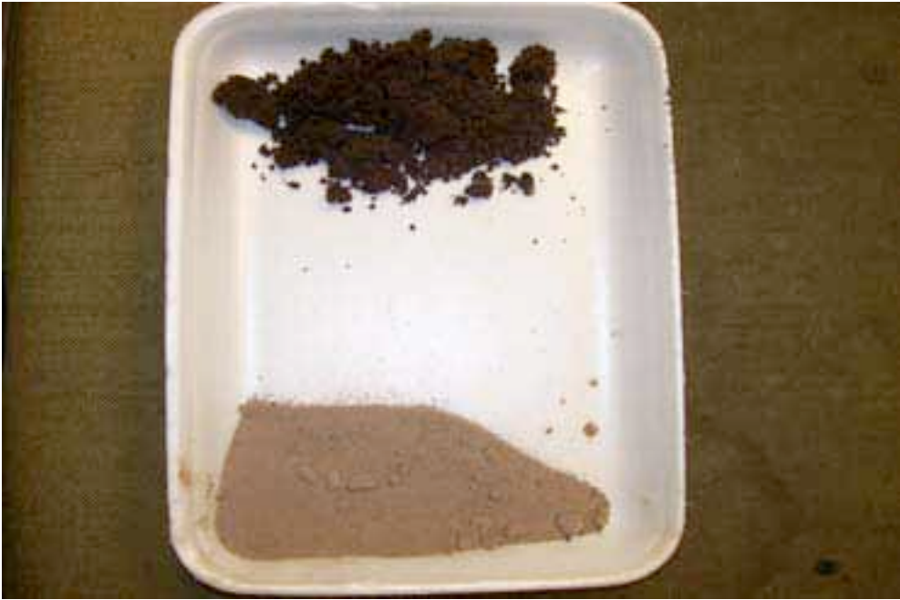
Figure 6.12. Top: Sand, clay, and water mixture before experiment. Bottom: residue after experiment.
